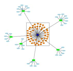
orange = map unit polygons, dark blue = single map unit key, green = component keys, light blue = horizon keys
